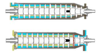
The principal feature of this system is the oil is extracted from the olive paste without the addition of water. Only if the olives happen to be too dry is 5% of water added, to reach the correct water content.
